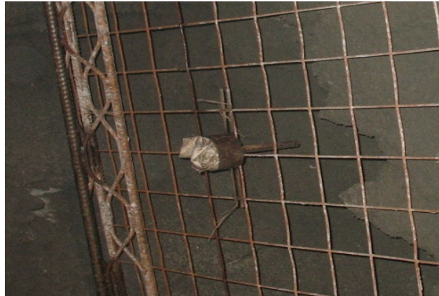
Figure 22: Dispositions of 3D targets in a tunnel profile
